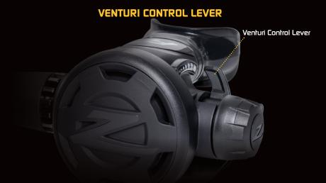
This lever controls the sensitivity of the regulator. The DIVE and PRE-DIVE Positions for the lever are marked on the case beside the lever. To avoid unexpected venturi free flows at the surface, or when entering into the water, the lever should be set in the PRE-DIVE **(forward)** position. As soon as the diver is ready to descend, the lever should be moved to the DIVE **(back)** position.
