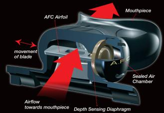
Atomic Aquatics has developed the first and only automatic flow control that automatically changes the breathing characteristics with depth. At depth, the air density increases (gets thicker) and it becomes harder to move through the regulator. The result is increased breathing effort at depth. Many regulators have different types of devices to increase flow (venturi) but these are either fixed in place or manually set and
