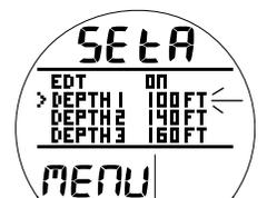
Fig. 104 - AJUSTE ALARMA PROFUNDIDAD 1 APNEA
