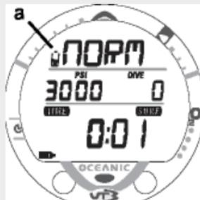
Fig. 2 - Low Battery Warning
