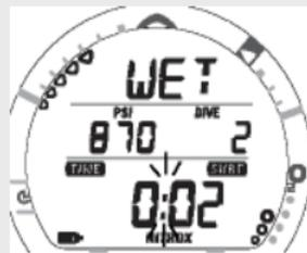
**Fig. 16 - NORM SURF MAIN (post dive, unit wet)**
