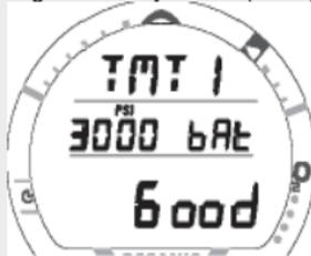
Fig. 5 - Transmitter 1 Battery Status (Good)
