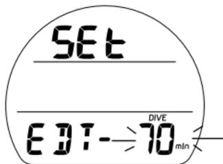
Fig. 22 - AJUSTE ALARMA EDT
