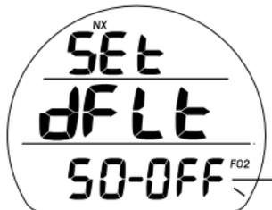
Fig. 18 - AJUSTE FO2 PRE-DETERMINADA
