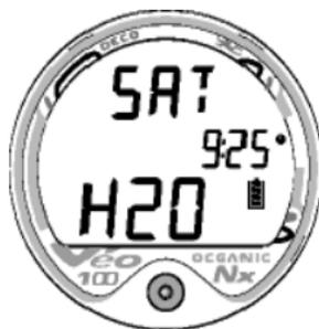
Fig. 61 - DESAT (unit wet)
