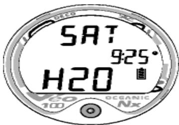
Fig. 61 - DESAT (unit wet)
