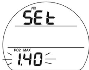
Fig. 27 - AJUSTE ALARMA
