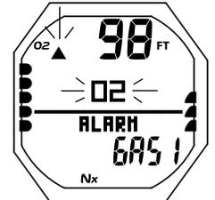
Fig. 98 - ALLARME O<sub>2</sub>ALTO (100%) PRINCIPALE
