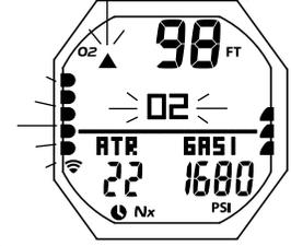
Fig. 105 - ALLARME O<sub>2</sub> ALTO (100%) PRINCIPALE
