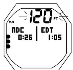
Fig. 140 - ALLARME DD
