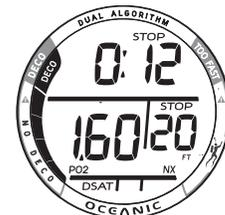
Fig. 41 - ALARME PO<sub>2</sub> EN PHASE DE DÉCOMPRESSION
