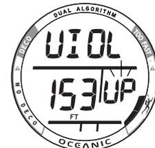
Fig. 37 - ÉCRAN PRINCIPAL D'INFRACTION AVEC LIMITATION AU MODE PROFONDIMÈTRE
