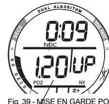
Fig. 39 - MISE EN GARDE PO<sub>2</sub>
