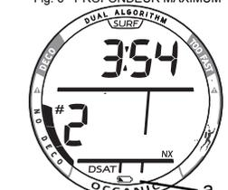
Fig. 7 - MISE EN GARDE DE PILE FAIBLE
