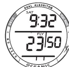
Fig. 14 - TEMPS D'INTERDICTION DE VOL/DE DÉSATURATION (FLY/DESAT)
