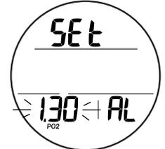
Fig. 57 - AJUSTE ALARMA PO<sub>2</sub>
