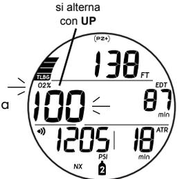
Fig. 115 - ALLARME O<sub>2</sub> PRINCIPALE (in curva)
