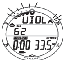
Fig. 102 - VIOLATION GAUGE DIVE MAIN
