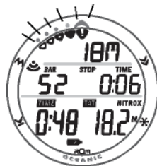
Fig. 100 - DELAYED VIOLATION #2 MAIN
