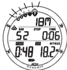
Fig. 100 - DELAYED VIOLATION #2 MAIN
