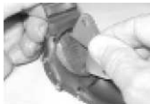
Fig. 144 - BATTERY HATCH REMOVAL (Tool)
