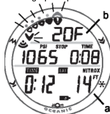
Fig. 98 - CONDITIONAL VIOLATION MAIN
