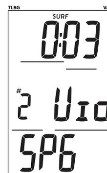
Fig. 70 - ÉCRAN PRINCIPAL SURFACE D'INFRACTION AVEC LIMITATION AU MODE PROFONDIMÈTRE
