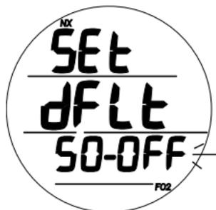
Fig. 44 - AJUSTE FO2 PRE-DETERMINADA
