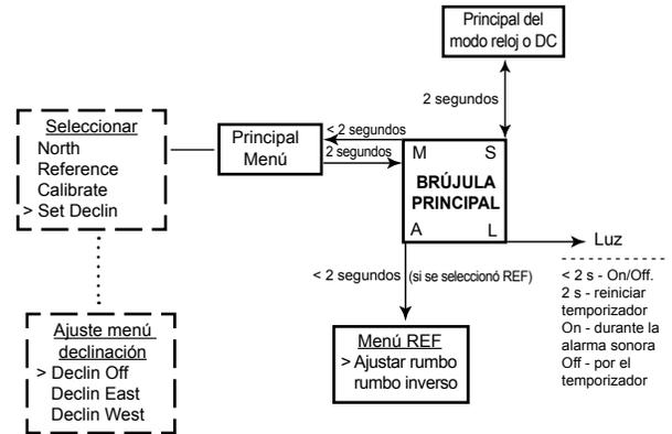
**ESTRUCTURA DEL MODO NORM SURFACE (NORMAL SUPERFICIE)**
