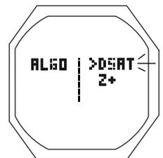
Fig. 47 - AJUSTE ALGORITMO
