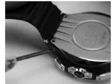
Fig. 179A - AFLOJAR TAPA DE LA BATERÍA
