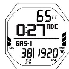
Fig. 63A - IMMERSIONE NORM (TLBG in curva)
