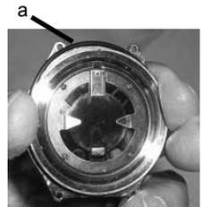
Abb. 181 - DECKEL-O-RING ZUSAMMENDRÜCKEN
