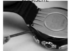
Abb. 179A - ZUM LÖSEN DES BATTERIEDECKELS
