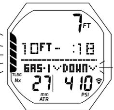
Fig. 86 - ÉCRAN PRINCIPAL D'INFRACTION DIFFÉRÉE 1 (pendant signal sonore)
