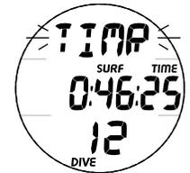
Fig. 61 - ALARMA CDT EN MODO FREE EN SUPERFICIE
