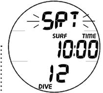
Fig. 62 - ALARMA SRT EN MODO FREE EN SUPERFICIE
