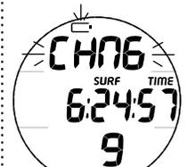
Fig. 64 - ALARME DE PILE FAIBLE EN SURFACE EN MODE FREE
