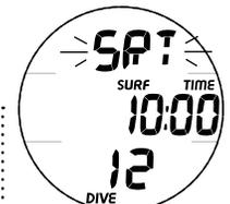
Fig. 62 - ALARME DE TEMPS DE RÉCUPÉRATION EN SURFACE EN MODE FREE
