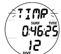
Fig. 61 - ALARME DU MINUTEUR DE COMPTE A REBOURS EN MODE FREE EN SURFACE
