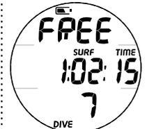
Fig. 63 - AVERTISSEMENT DE PILE FAIBLE EN SURFACE EN MODE FREE
