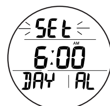
Fig. 22 - DAILY ALARM STATUS (Set, ready)
