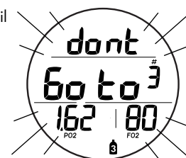
Fig. 120 - GAS SWITCH WARNING
