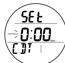
Fig. 14 - SET CDT (after access from Status)
