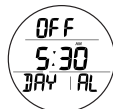
Fig. 20 - DAILY ALARM STATUS (to access Set)
