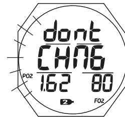
Fig. 93 - GAS SWITCH ALARM (all flash)
