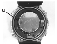
Fig. 136 - RELEASE BATTERY TERMINAL
