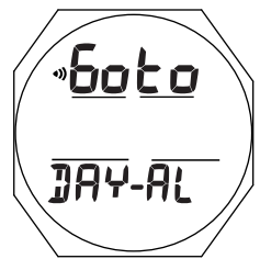
Fig. 12 - DAILY ALARM LEAD-IN
