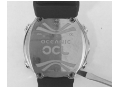
Fig. 134 - TO LOOSEN BATTERY COVER
