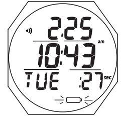
Fig. 2 - WATCH MAIN (low battery alarm)
