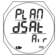
Fig. 29A - PLAN LEAD-IN (Gas 1 set for Air)
